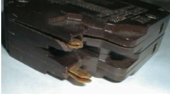
Figure 8 – Damaged “E” type breaker
